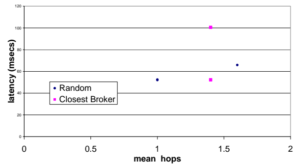
Fig. 8 Mean event delivery hops versus delivery latency
