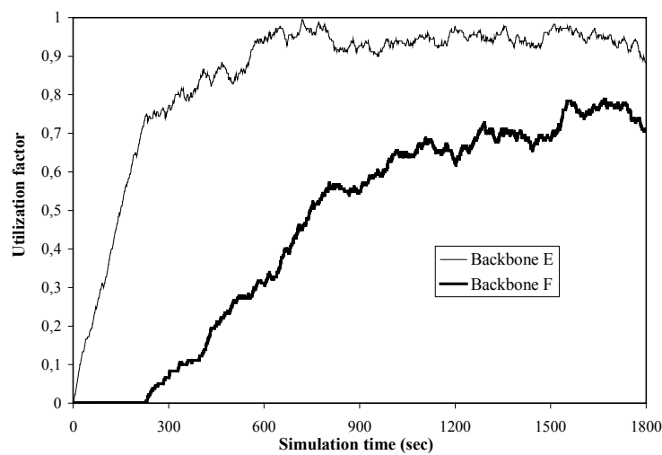
Fig. 21 - Utilization factor of backbone domains: very heavily loaded case and MB inter-domain routing algorithm.
